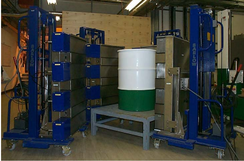
Fig. 2. Configuration of DISPIM ® Imaging System drum measurements
