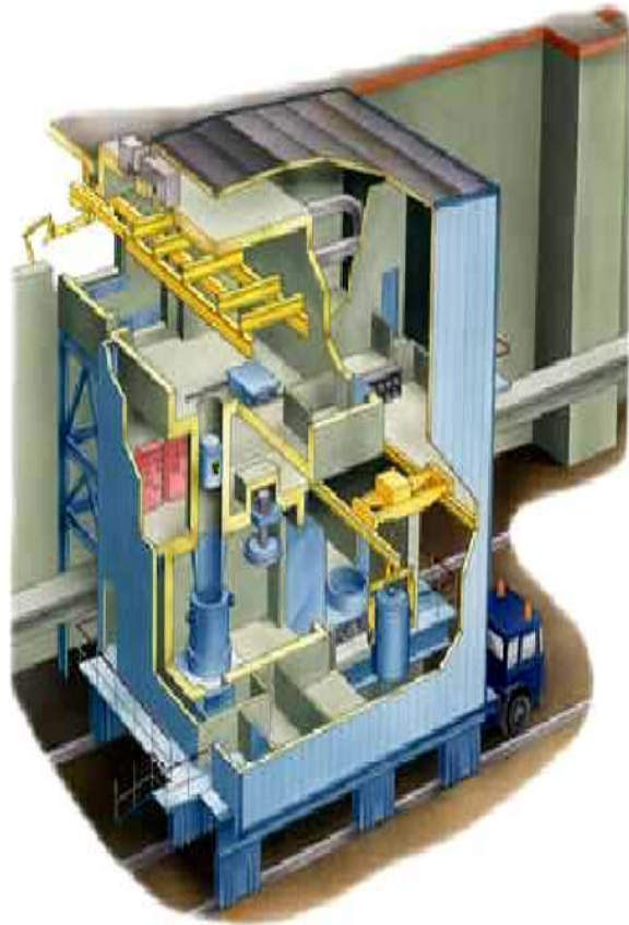
Fig. 2. Mobile Decommissioning Module
