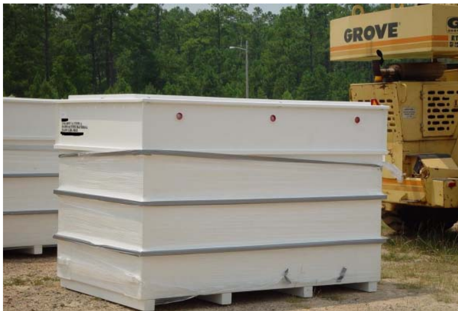
Fig. 2. Standard large box (SLB-2); the payload container for the TRUPACT-III
