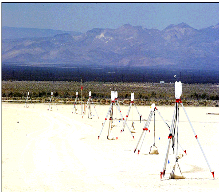
Fig. 2. Portion of PID array located downwind from stack at the NTS
