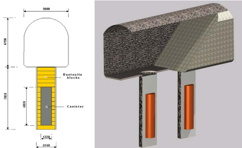
Fig. 4. View of the closed disposal holes and the backfilled disposal tunnel.
