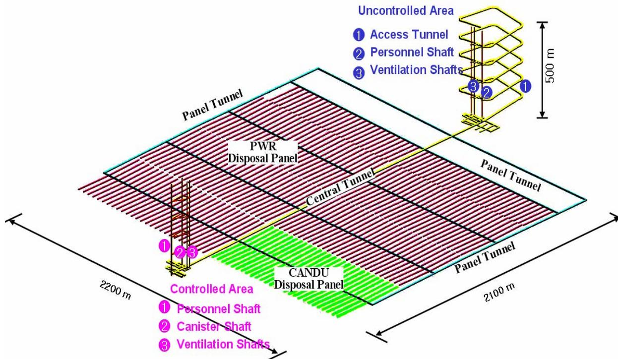
Fig. 2. Layout of the Korean reference HLW Vertical disposal system.
