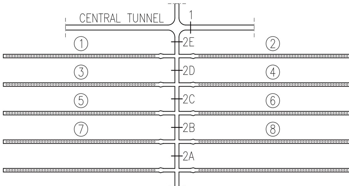
Fig. 3. First operation in the CANDU tunnels of the repository.
