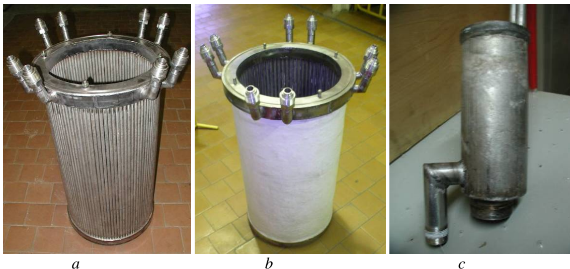
Fig. 1. View of the 418 mm inner diameter CCIM as manufactured (left), coated with a protection layer (middle), and pouring unit (right).
