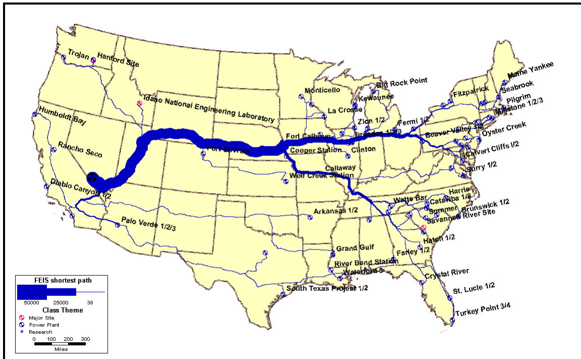
Fig. 1. Shipments to Yucca Mountain over 24 years, mostly truck scenario, using representative routes identified in the DOE FEIS
