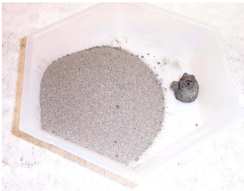
Fig. 2. Bed material and nozzle deposit formed during operation with the MAC/DTPA feed
