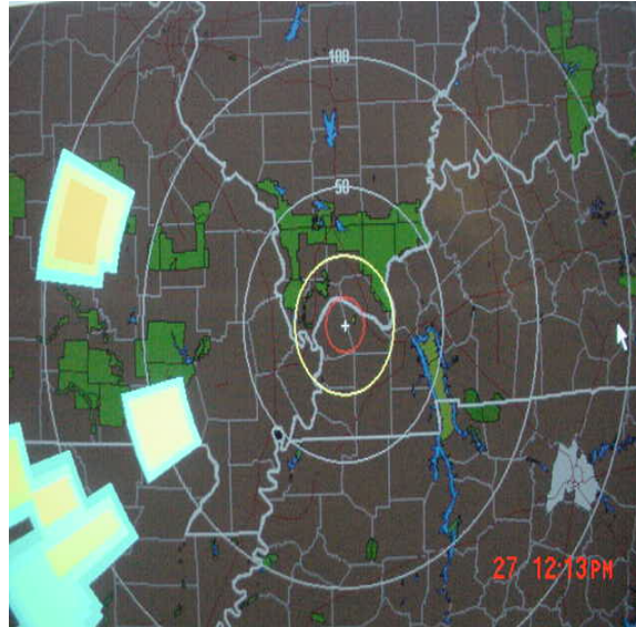
Fig. 12. Color-coded storms traveling in the same direction for longer than one minute
