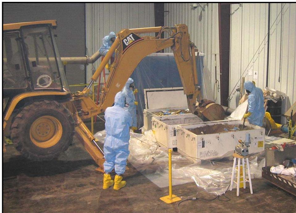
Fig. 4. Loading Rocky Flats mixed DU waste into ICV container for GeoMelt processing
