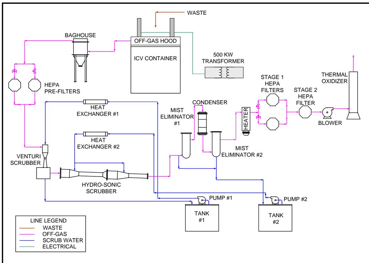
Fig. 1. GeoMelt pilot-scale system process flow diagram
