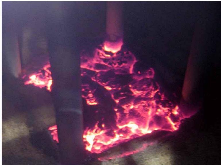
Fig. 8. Mock HE melt surface during operations.
