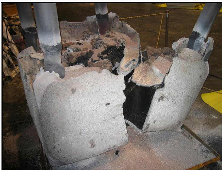
Fig. 3. Vitrified monolith from TSCA mixed waste melt 2
