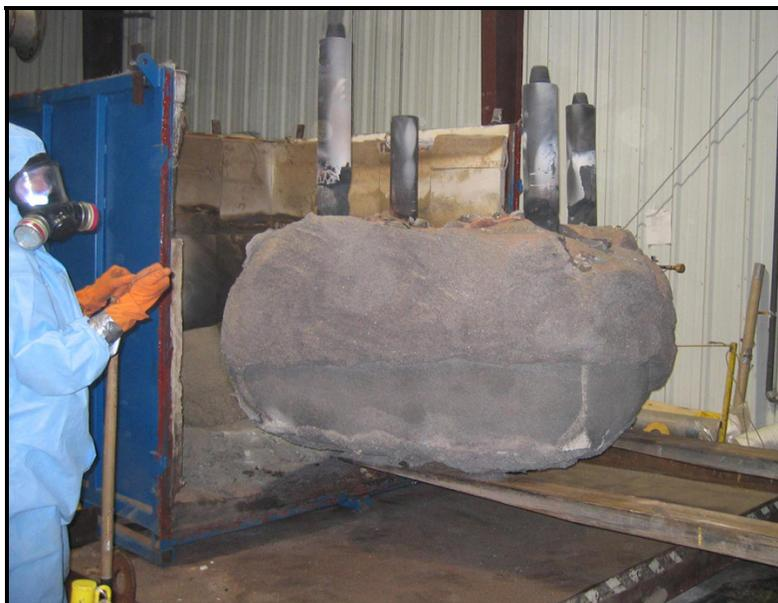
Fig. 5. The Rocky Flats DU mixed waste melt 1 vitrified monolith
