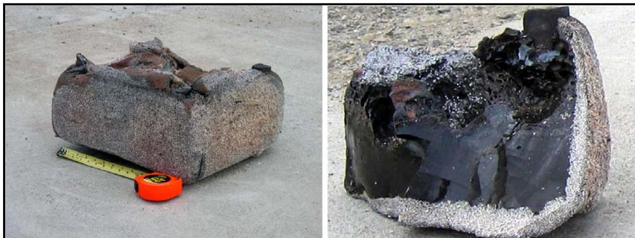
Fig. 9. The Sandia Mock HE vitrified block (left) and after it was fractured for sampling (right).
