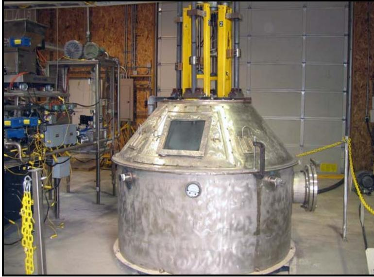
Fig. 7. Engineering-scale ICV test container
