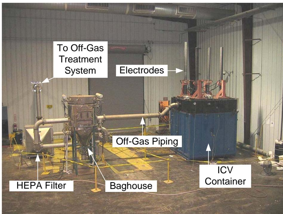
Fig. 2. GeoMelt pilot-scale ICV container and initial off-gas treatment components
