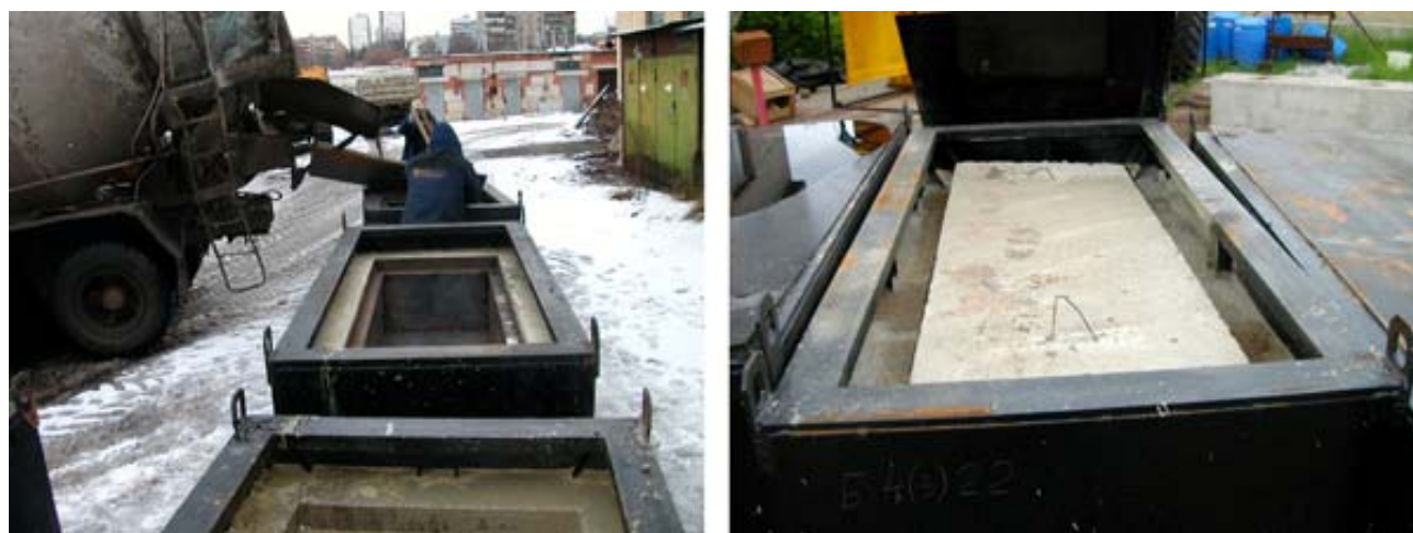
Fig. 3. Reinforced metal containers with concrete inserts (a) and concrete lids (b)
