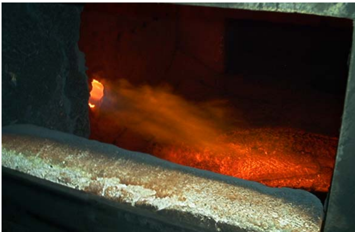
Fig. 2. Inside of a BPU burn chamber this picture depicts EDTA mixing with natural gas flame and residual inorganic material collection.
