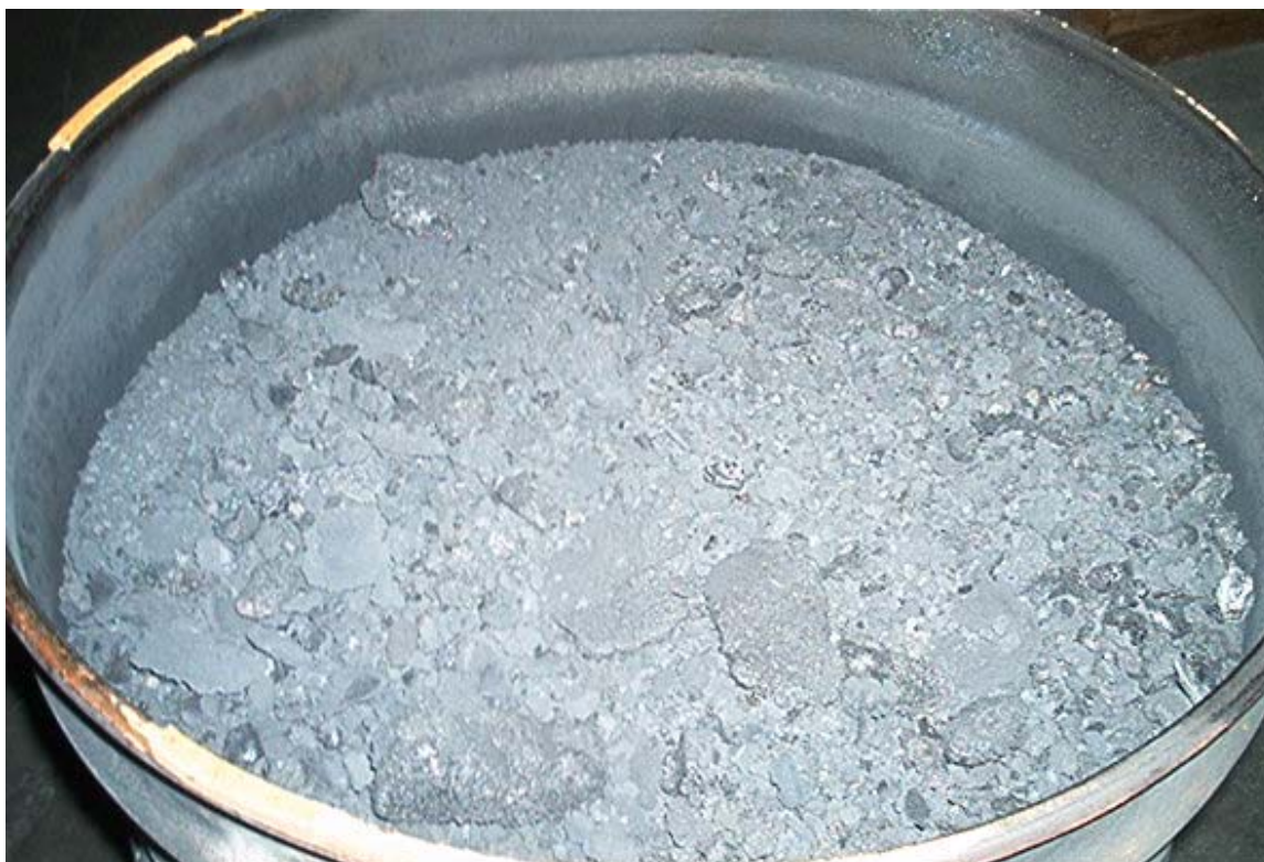
Fig. 3. Residue from thermal treatment of EDTA liquids
