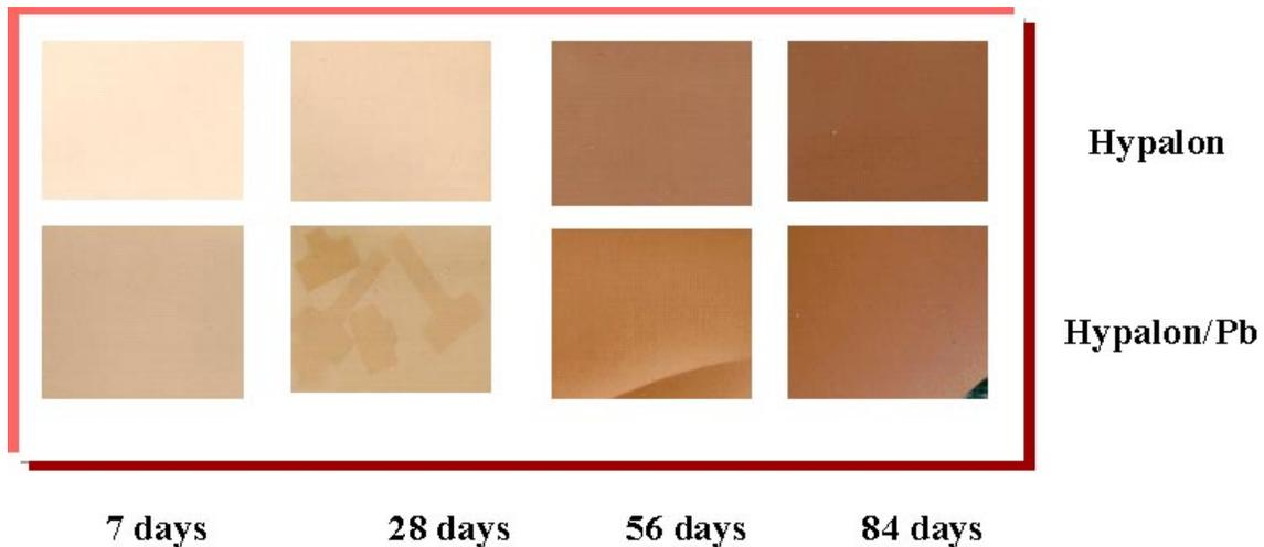
Fig. 3. Color change correlates with Hypalon material heated at 120°C.
