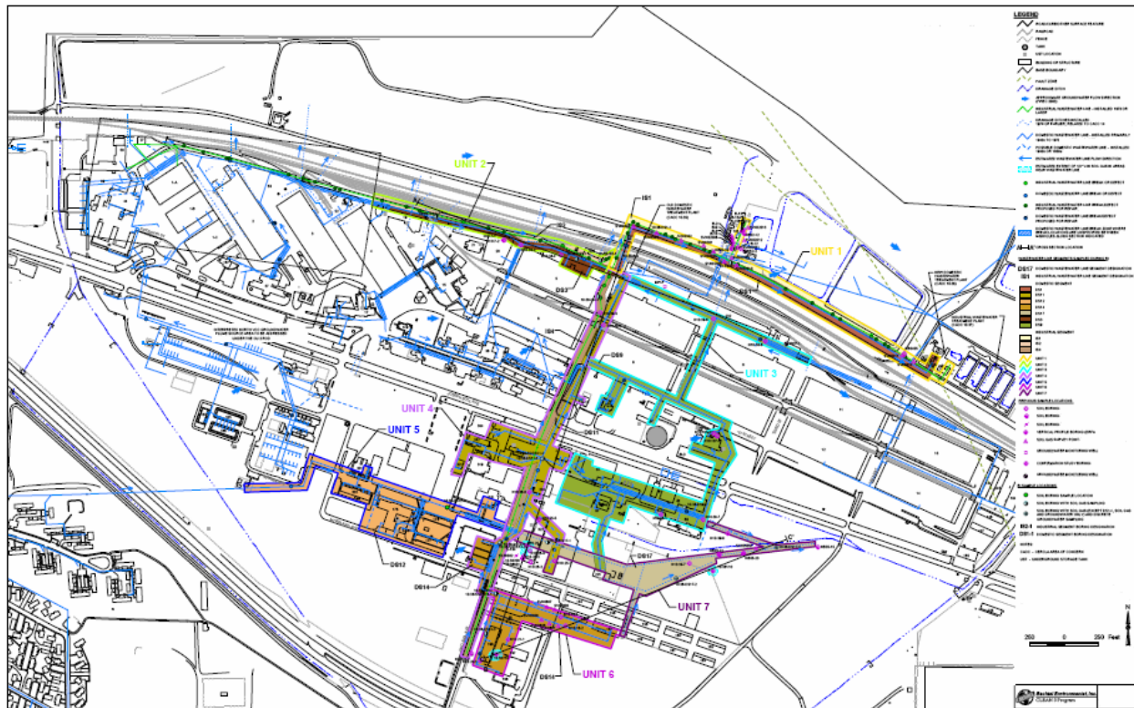
Fig. 3. Unit designations for wastewater collection lines
