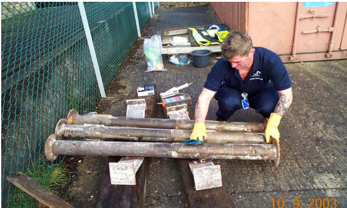
Fig. 2. Typical steel lined penetrations recovered from cave line blocks being monitored in controlled area of external compound
