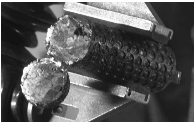
Fig. 4 Sectioned basket of spent oxide fuel reduced to metal.
