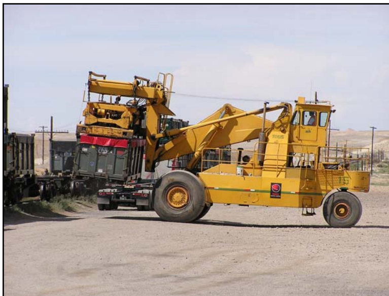
Fig. 3 Off-loading an intermodal container at the MHF-LS Cisco trans-load facility.
