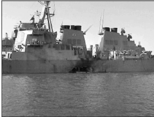
Fig. 1 Blast damage to USS Cole by Watercraft bomb
