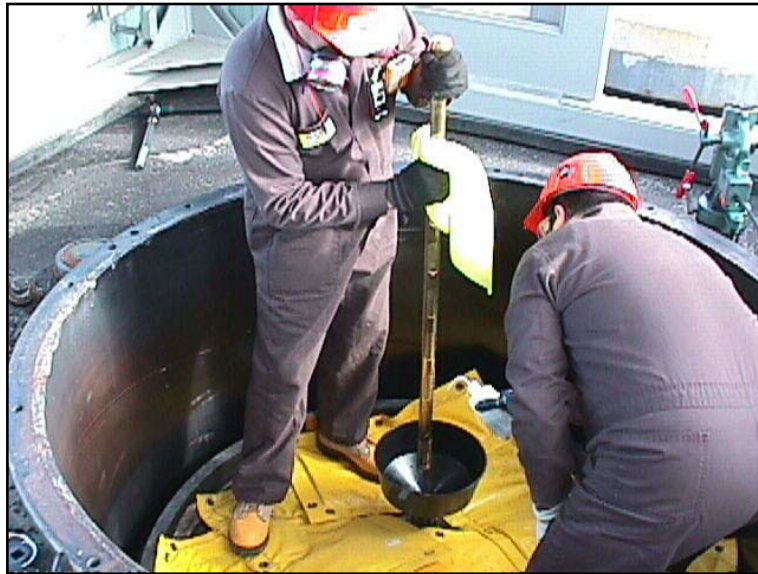
Fig. 2 Resin sampling from a liner stored within an in-ground container
