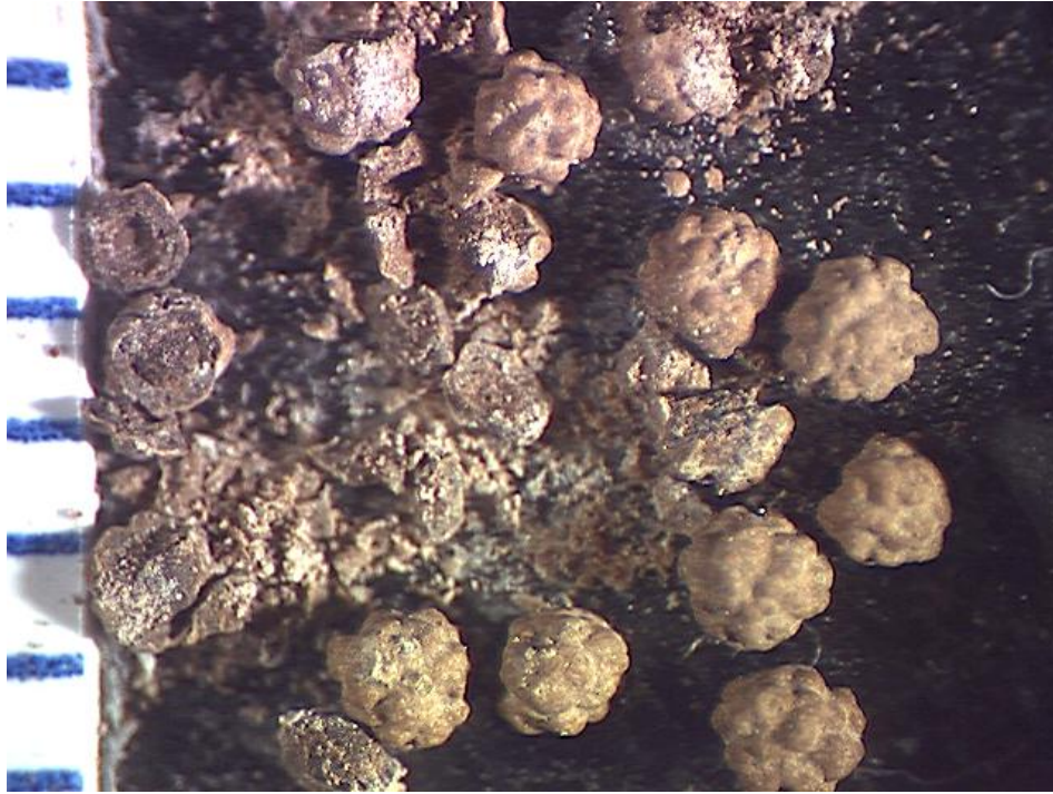
Fig. 3 Optical Micrograph of Sodium Carbonate Bed Product Particles. Blue Marks at the Left Indicate Scale (1 mm Between Marks). Some particles are crushed to show the Inner Core of Starting Bed Media.
