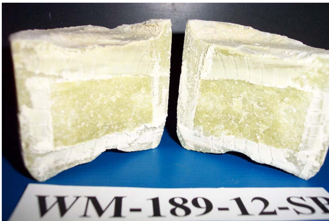
Fig. 2 Picture showing nature of flask-scale product (saw and chisel marks required for breaking in half).
