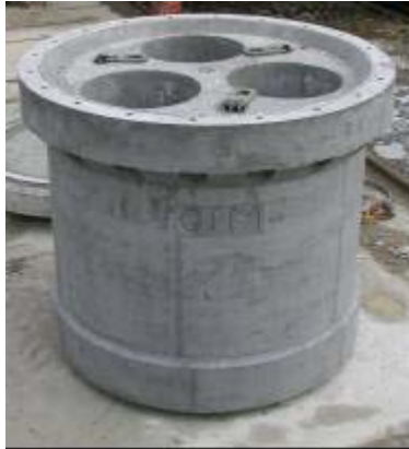
Fig. 4 Example of a long-lived intermediate-level waste container
