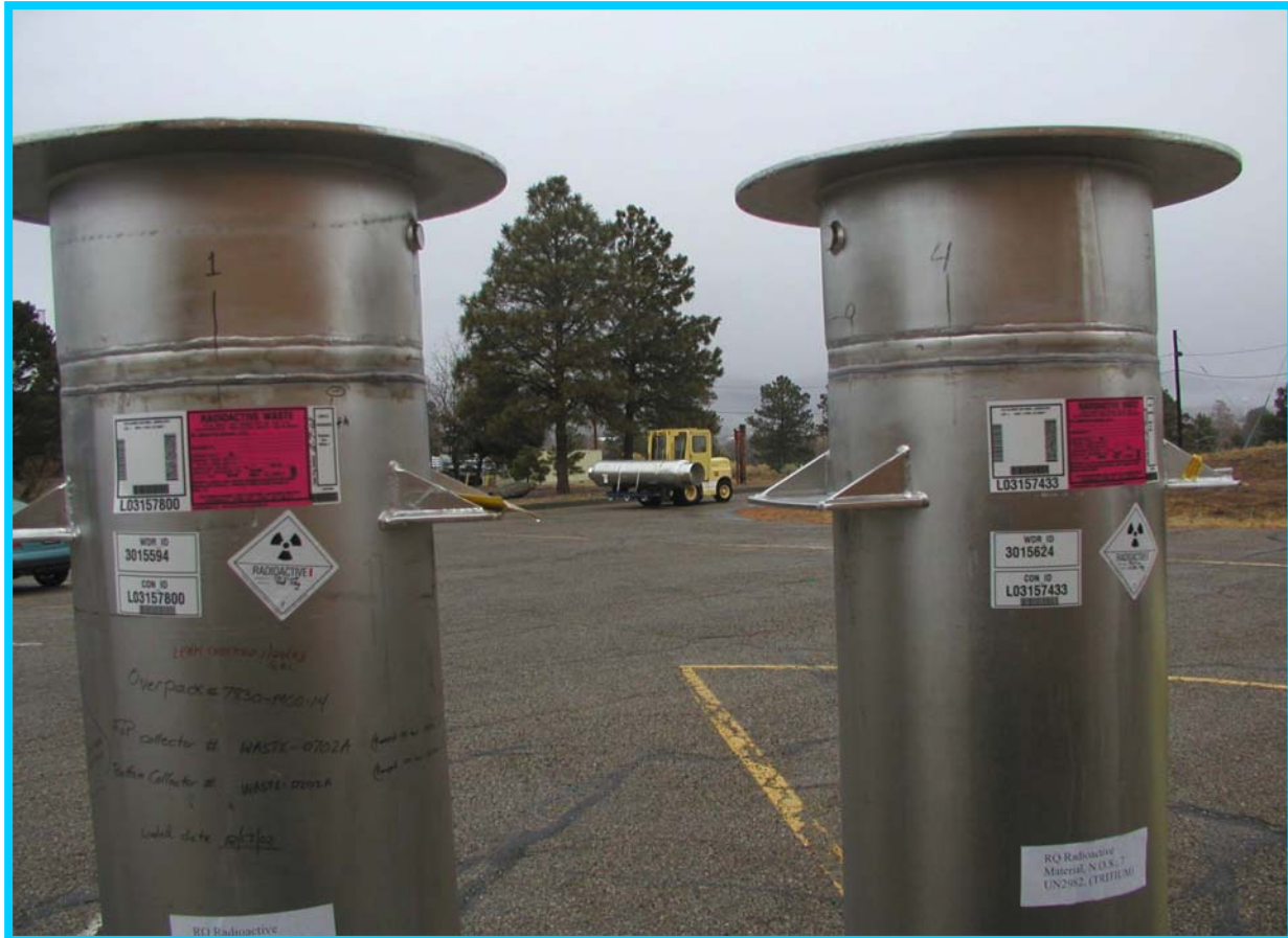
Fig. 4 Overpack Waste Containers Containing Moisture Collectors
