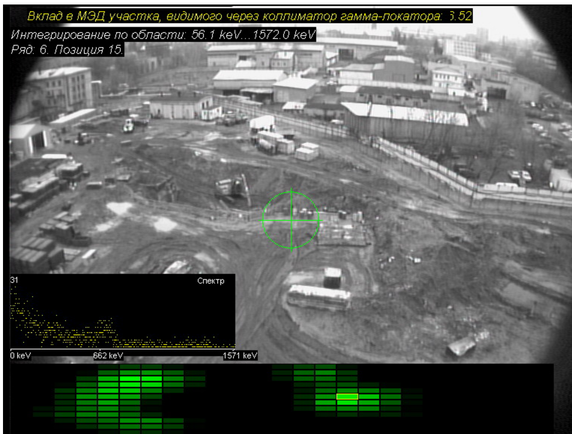
Fig. 2 Presentation of primary data, obtained with gamma-locator
