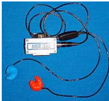
Fig. 2 EarMic system showing right and left ear pieces and push-to-talk button.
