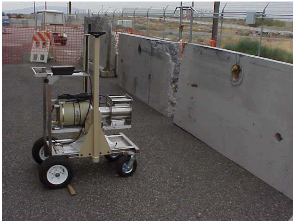
Fig. 4 Building debris being verified as clean with the field HPGe assay unit
