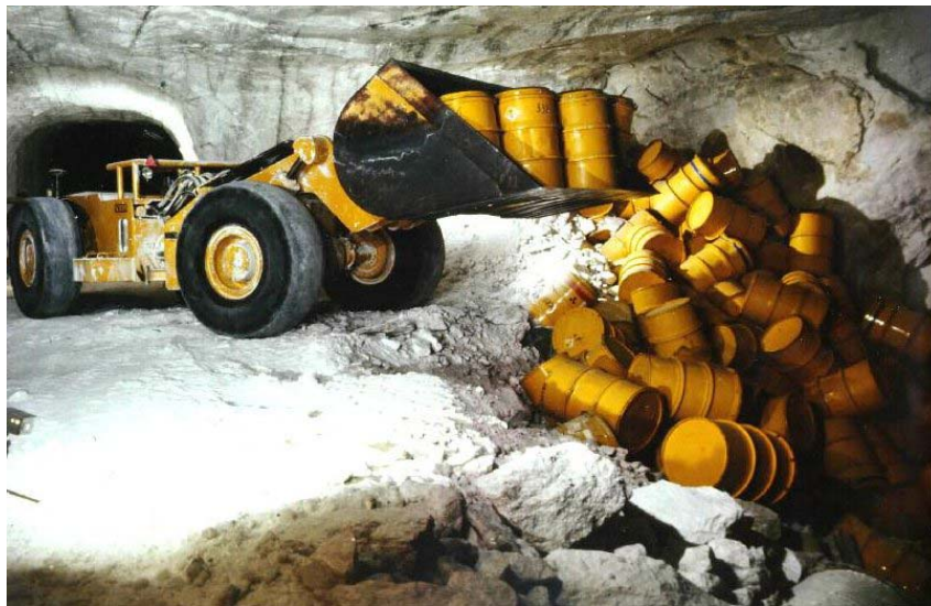
Fig. 3 LLW disposal by drop-down technique
