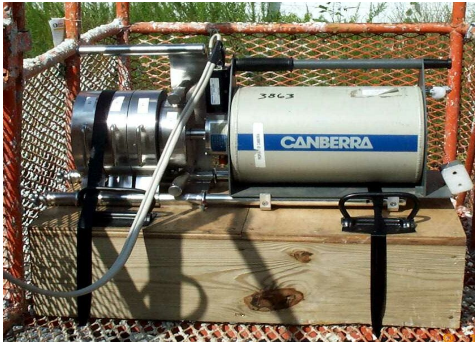
Fig. 2 ISOCS detector mounted in the basket of the 80-foot boom
