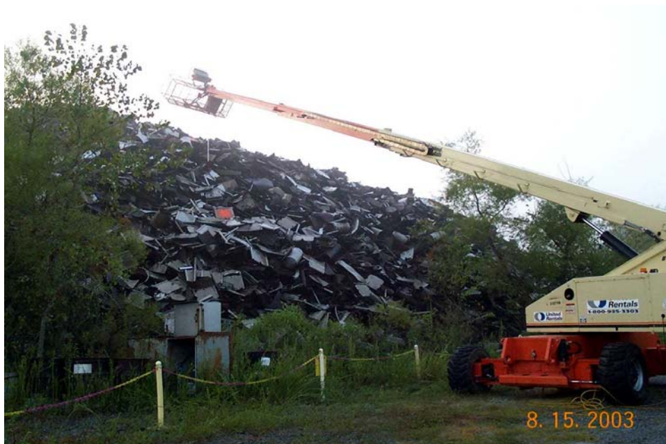
Fig. 3 Photograph of ISOCS detector deployed in boom basket over the 16a steel pile
