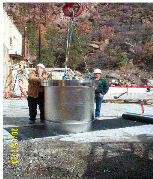
Fig. 1 Handling a specially designed pressure vessel for the packaging of an 8,000-curie beryllium reflector
