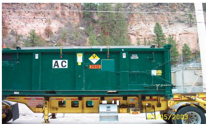
Fig. 2 Intermodal container used for the packaging and transport of bulk LLW.
