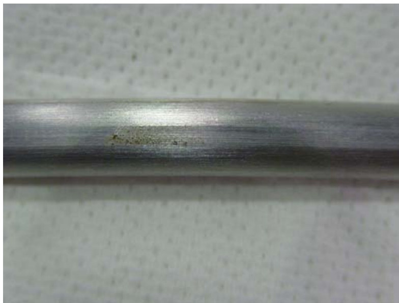
Fig. 1 Pitting scars on the aluminum coated seal of the Primary Lid
