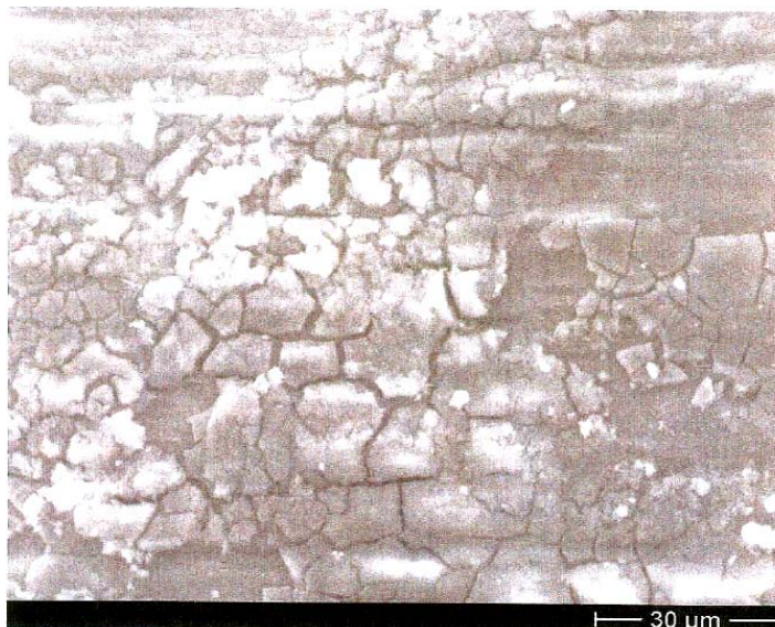
Fig. 2 SEM picture at the place of pitting corrosion of the aluminum seal
