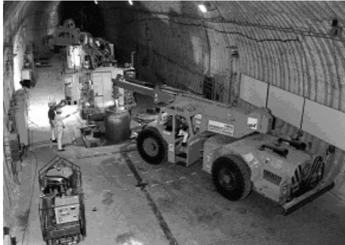
Fig. 3 Testing of a HLW disposal system / concept in the Asse mine / URL.
