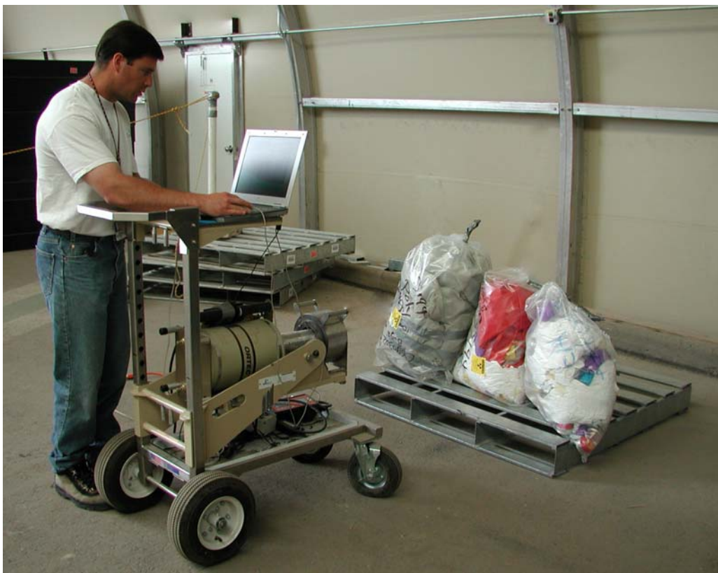
Fig. 4 HPGe measurement of secondary DVRS waste
