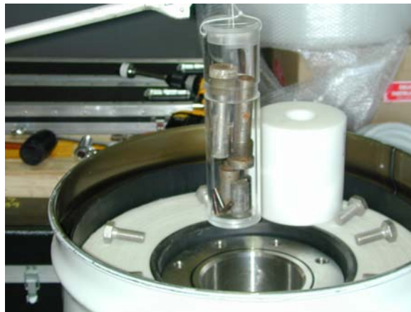
Fig. 3 Excess americium-241 neutron source prepared for loading in the S-100 multifunction container.
