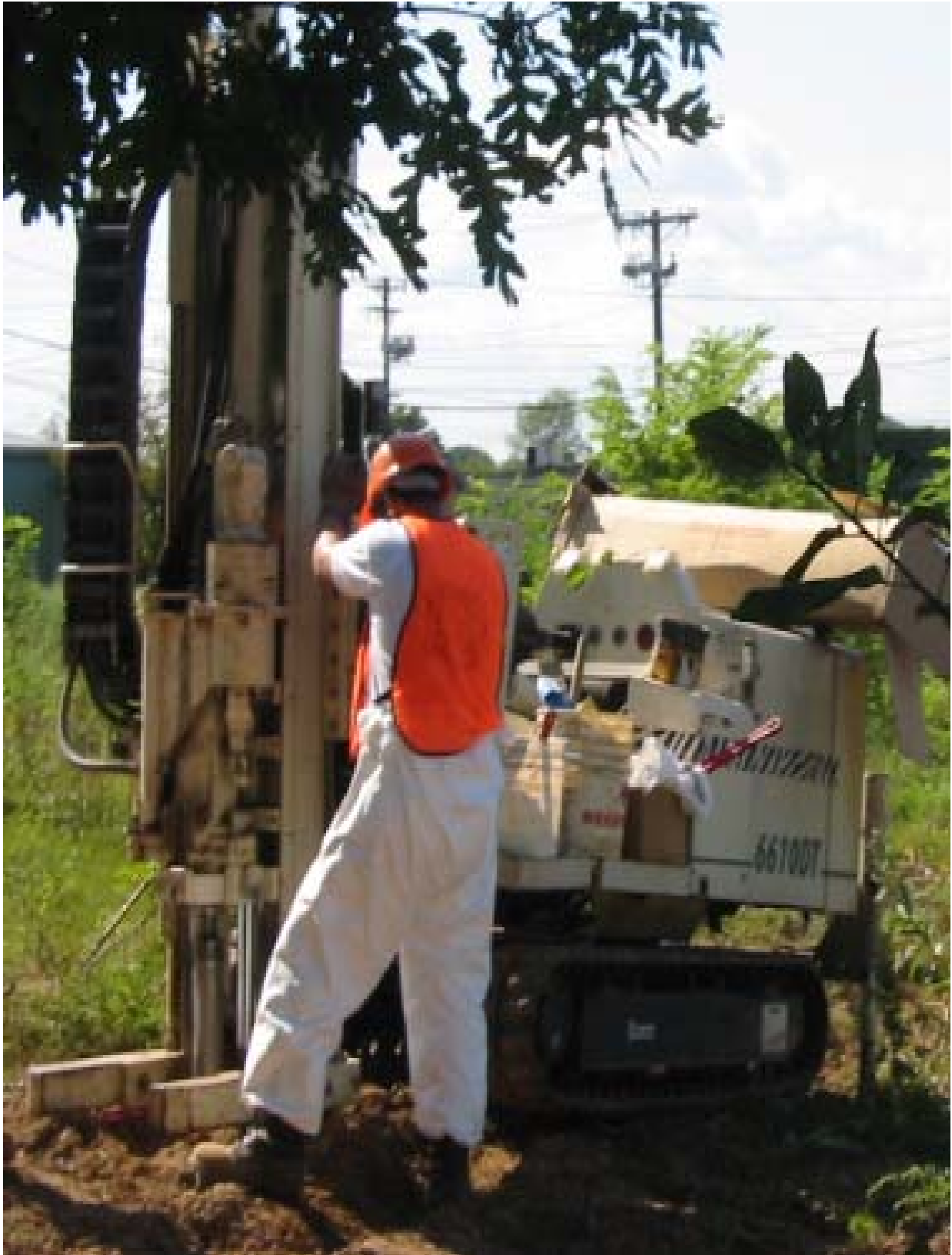
Fig. 3 Example of direct push equipment
