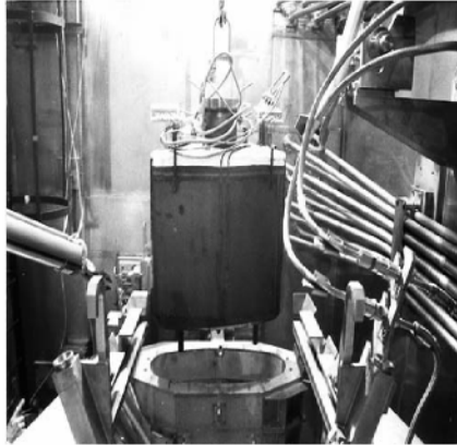
Fig. 3 Melting pot transfer from the melter to the dismantling cell
