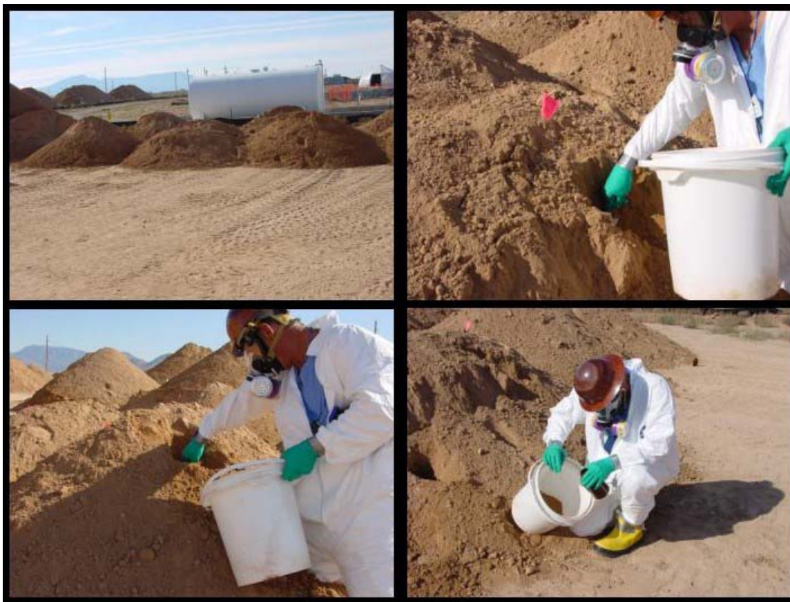
Fig. 2 Segmenting and sampling soil piles for tritium as a waste minimization effort
