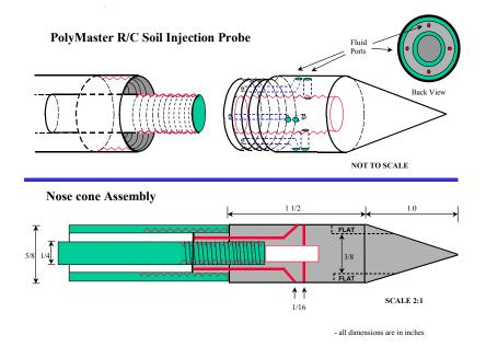
The resin and catalyst are separated by an inner and outer casing and mix immediately on exit from the soil probe. The injection angles are designed such that material is delivered laterally in a 360 degree angle around the probe.
