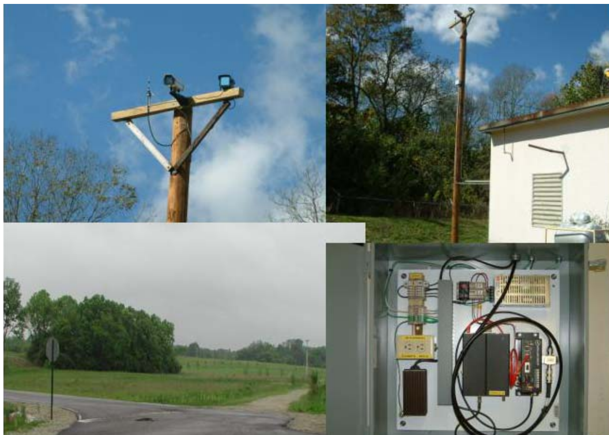
Fig. 3 Machine vision system with infrared illuminator monitoring for soil removal
