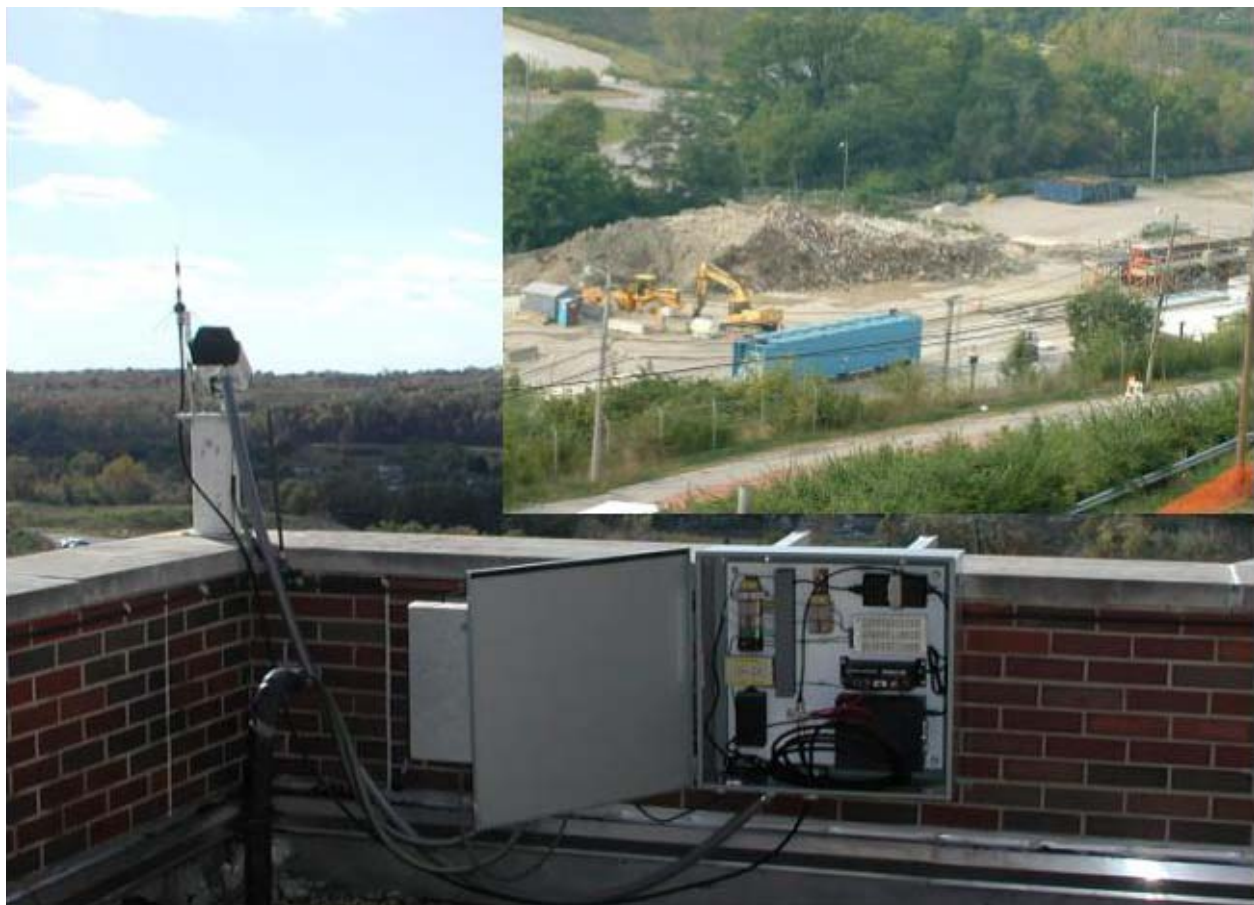
Fig. 1 The machine vision system monitoring the waste-soil-stockpile facility
