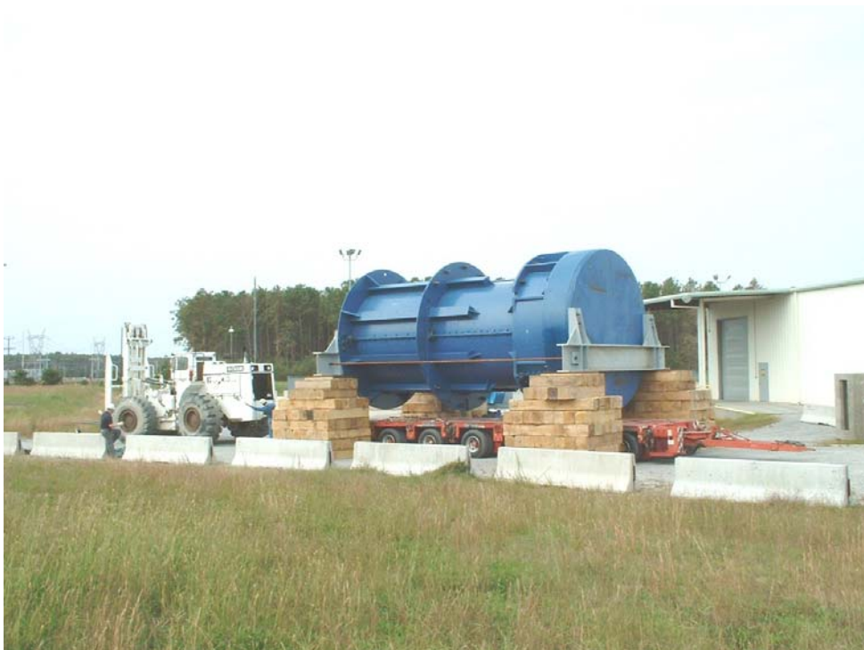
Fig. 4 WMG Intact Vessel Head Transport System
