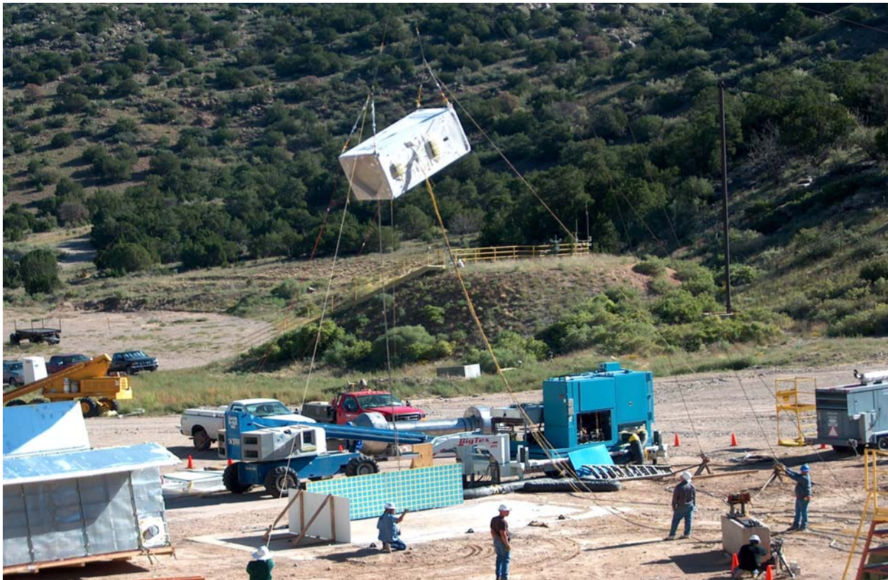
Fig. 2 9-m free drop of the TRUPACT-III package – lid slapdown orientation
