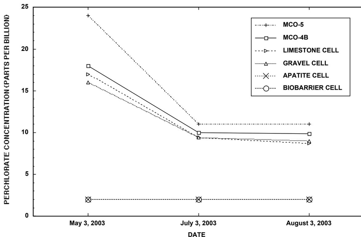
Fig. 4 Concentration of perchlorate in groundwater samples collected from up- (MCO-4B) and down-gradient (MCO-5) monitor wells and reactive media cells during three different sampling events. During construction in February 2003, the concentration of perchlorate in alluvial groundwater was 35 ppb.
