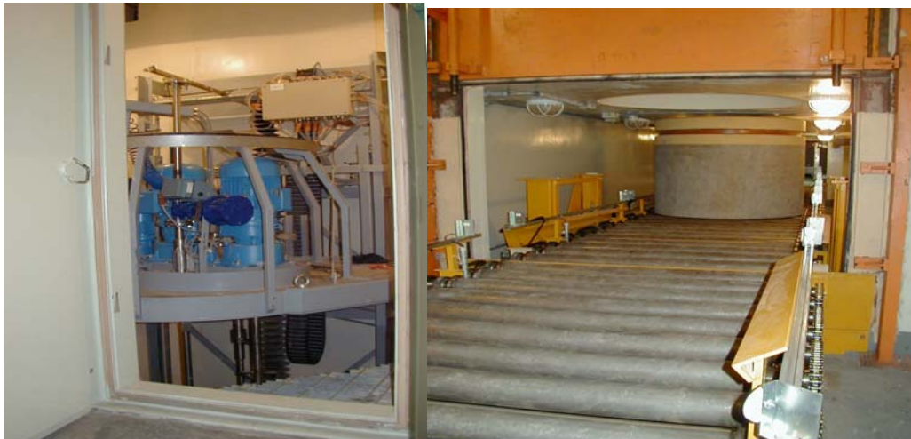
Fig. 4 In-cask mixer on the left and docking position underneath the mixer on the right
