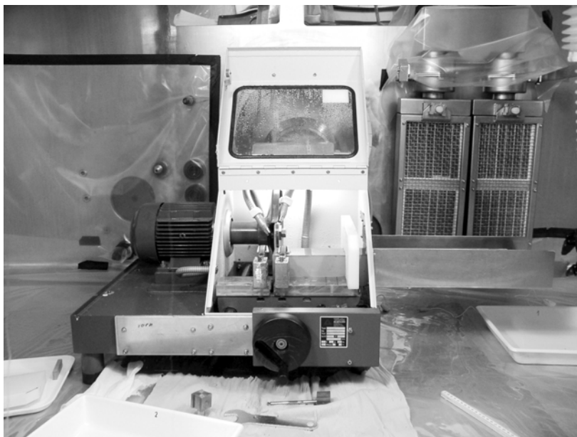
Fig. 3. Installation of a low-speed diamond saw in the RCM hot cell facility for the destructive sampling of the selected beryllium element no. 21.
