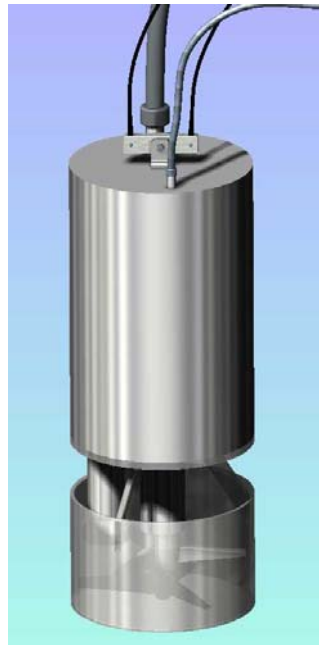
Fig. 1 The mixing and pumping module of the CSR system
