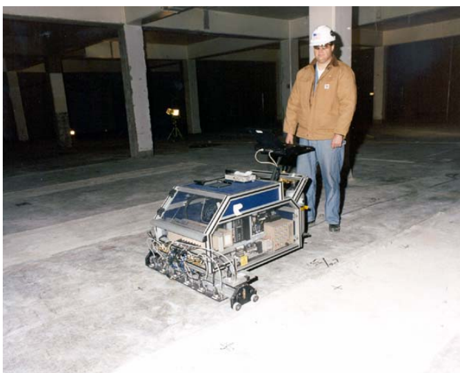
Fig. 1 A Radiological Control Technician demonstrates the final survey monitor in an uncontaminated area
