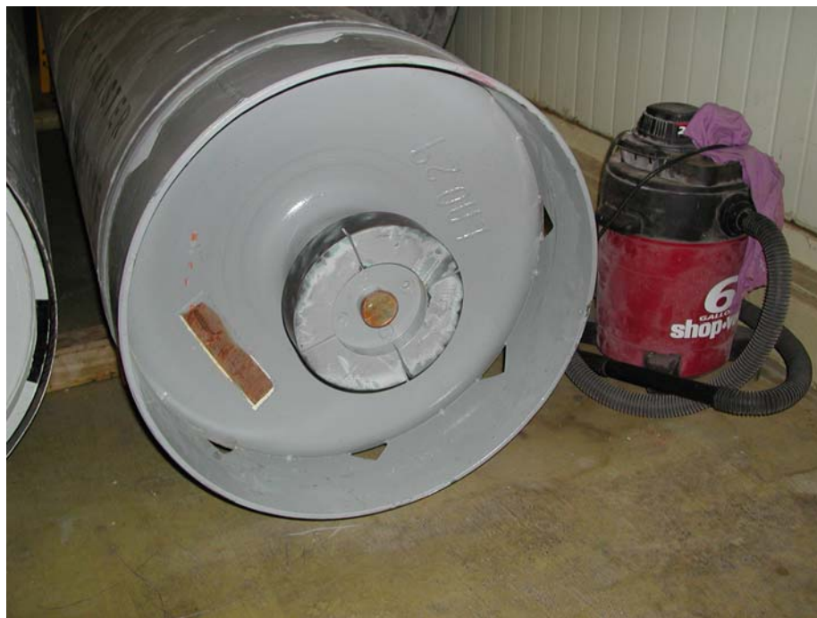
Fig. 1 Horizontal welded RH-TRU waste container
