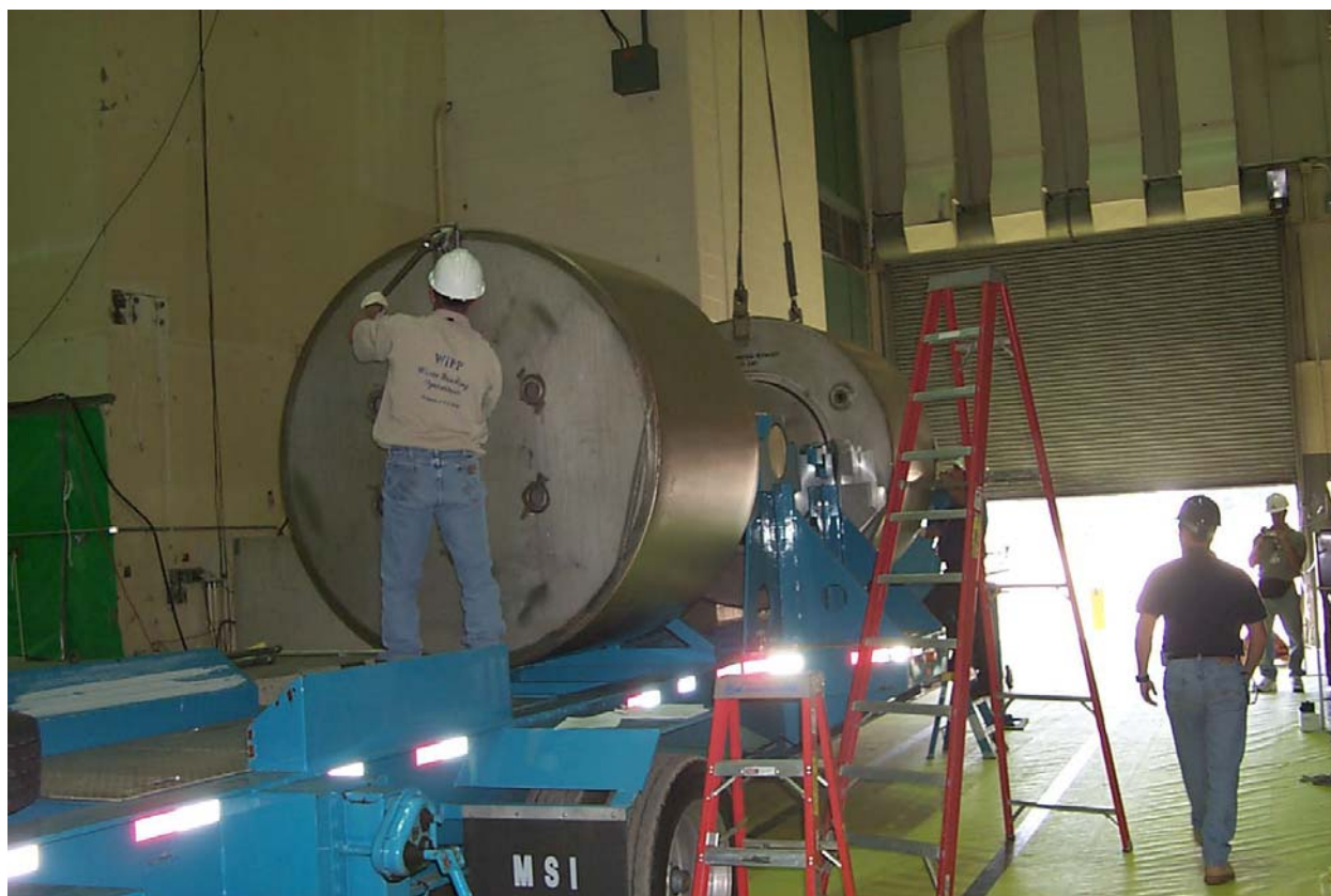
Fig. 3 WIPP 72-B cask with impact limiters on shipping trailer
