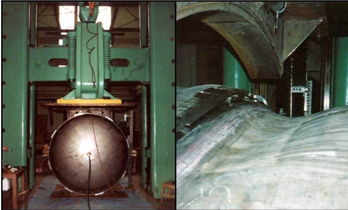
Fig. 3 Compression testing of a full-scale TRUPACT-II package closure design
