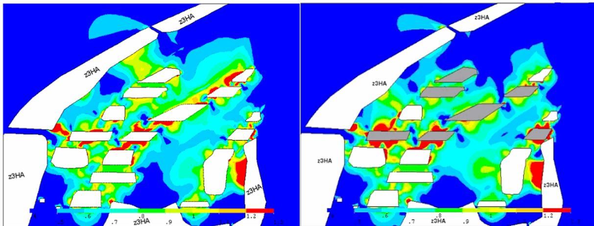
Fig. 3 Stress regimes (dilatancy boundary 1.0) before (A) and after (B) backfilling of the excavations (central part). The yellow, orange, and red areas mark a violation of the dilatancy criterion. Back-filled openings are marked dark gray (salt concrete).
