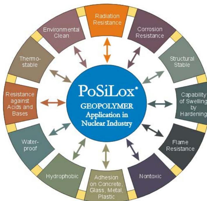
Fig. 1 Main properties of tailor-made Polysiloxane materials (some properties can be changed in a wide range)
