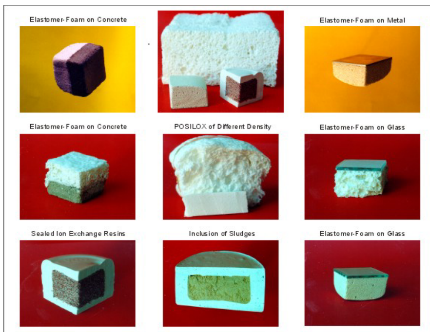
Fig. 2 Different application forms of Polysiloxane samples (rigid, flexible; film, foam, coating, encapsulation, conditioning)
