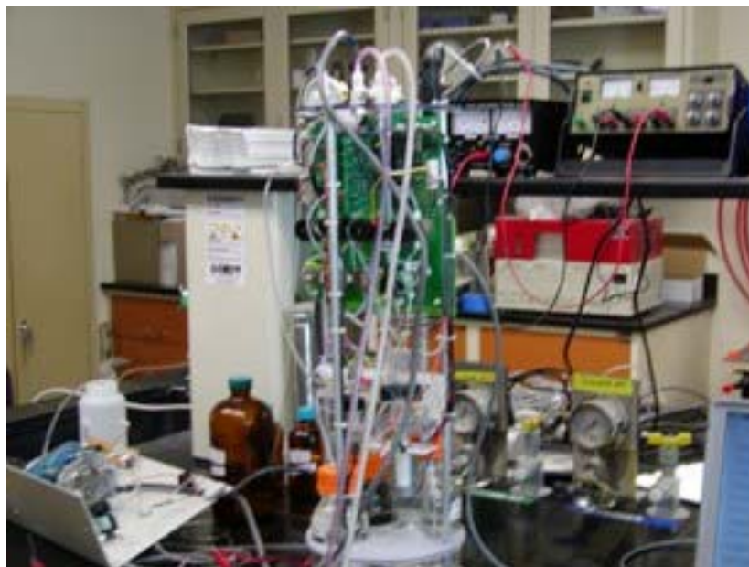
Fig. 3. The Chromium (VI) Sensor Platform Destined for the Columbia River Salmon Spawning Beds.
